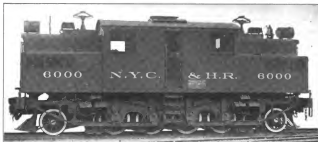
Fig. 4586. Electric Locomotive for the New York Central & Hudson River. Built by the General Electric and American Locomotive Companies.
